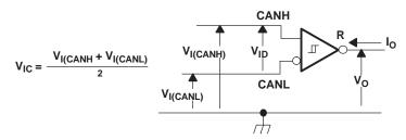
Figure 5. Receiver Voltage and Current Definitions
