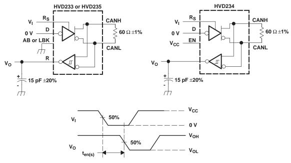
NOTE: All V<sub>I</sub> input pulses are supplied by a generator having the following characteristics:  $t_r$  or  $t_f \le 6$  ns, pulse repetition rate (PRR) = 125 kHz, 50% duty cycle.
