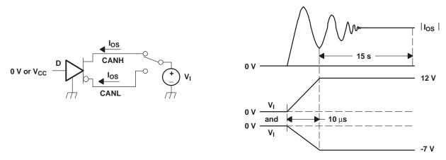
Figure 15. I<sub>OS</sub> Test Circuit and Waveforms
