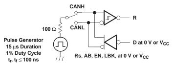
NOTE: This test is conducted to test survivability only. Data stability at the R output is not specified.
