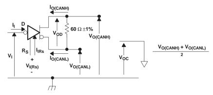
Figure 1. Driver Voltage, Current, and Test Definition
