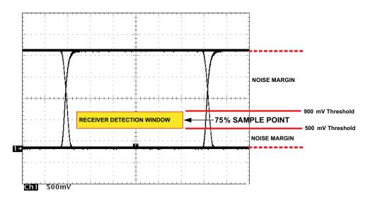
Figure 29. Typical SN65HVD230 Differential Output Voltage Waveform
