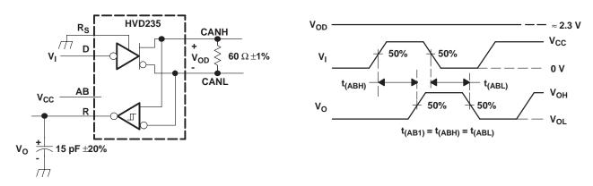
NOTE: All V<sub>I</sub> input pulses are supplied by a generator having the following characteristics:  $t_r$  or  $t_f \le 6$  ns, pulse repetition rate (PRR) = 125 kHz, 50% duty cycle.
