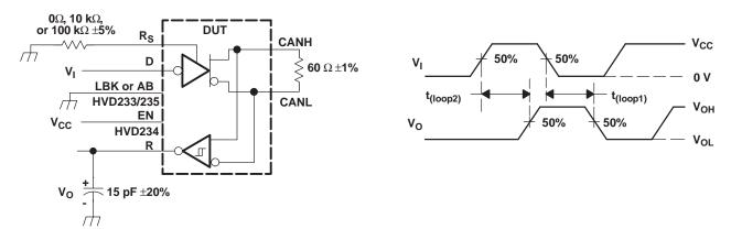
NOTE: All V<sub>I</sub> input pulses are supplied by a generator having the following characteristics:  $t_r$  or  $t_f \le 6$  ns, pulse repetition rate (PRR) = 125 kHz, 50% duty cycle.
