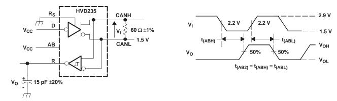
NOTE: All V<sub>I</sub> input pulses are supplied by a generator having the following characteristics:  $t_r$  or  $t_f \le 6$  ns, pulse repetition rate (PRR) = 125 kHz, 50% duty cycle.
