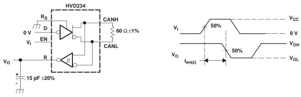
NOTE: All V<sub>I</sub> input pulses are supplied by a generator having the following characteristics:  $t_r$  or  $t_f \le 6$  ns, pulse repetition rate (PRR) = 50 kHz, 50% duty cycle.
